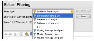
The Butterworth filter set is effectively a 6th order Butterworth filter. It is implemented by cascading a first-order and second-order Butterworth filters in the forward direction, then repeating in the backward direction. The performance of this filter was validated with numerous profile data including those from the FHWA 2004 Profiler Roundup.
