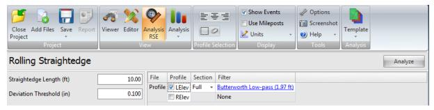
A different wavelength filter can be specified for each file by clicking the hyperlink for each input field. A pop-up dialog box would appear to allow you to select filter settings.
