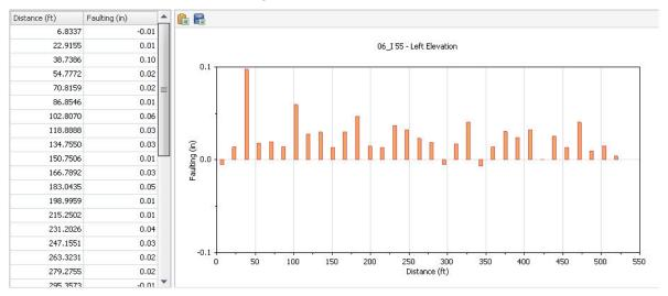
Select the top-level profile to show the maximum faulting and accumulated faulting for each segment.
